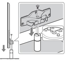
**2** Attach the TV and Table-Top Stand with the supplied screw and hexagon wrench.
